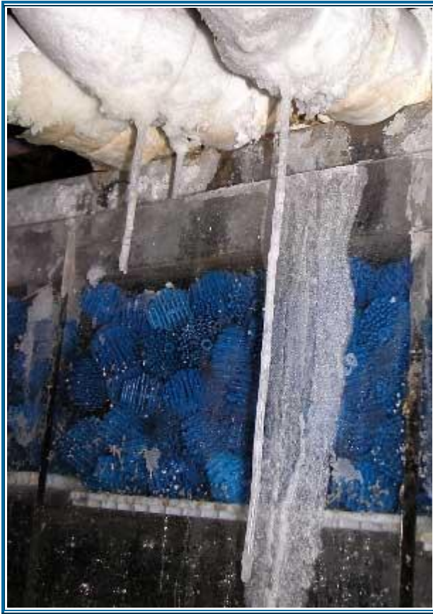
Figure 1. Salt creep is one way that salinity can change over time. This extreme case was captured in a photo by Bob Bottini (aquababy) owner of Tanks alot!
